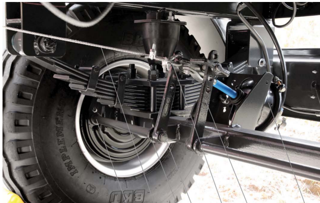
Fig. 6. Braking system components: 1 – brake shoe expander shaft; 2 – expander shaft lever (arm); 3 – arm adjusting comb on the expander shaft; 4 – lever adjustment nut on the expander shaft; 5 – the link (follower) that couples the pneumatic actuator rod with the expander shaft lever; 6 – parking brake cable; 7 – membrane actuator.
